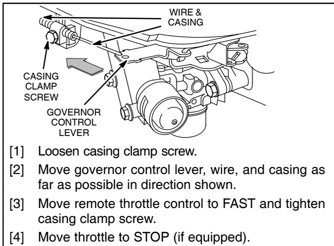
\* On some models the governor lever is fixed into position and is not adjustable.
