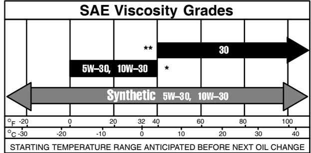
\* **CAUTION:** Air cooled engines run hotter than automotive engines. The use of non-synthetic multi-viscosity oils (5W-30, 10W-30, etc.) in temperatures above 40° F (4° C) will result in higher than normal oil consumption. When using a multi-viscosity oil, check oil level more frequently.
