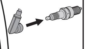
Make sure the spark plug boot is connected to the spark plug before attempting to start.
