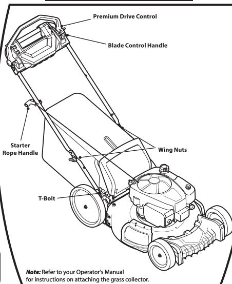
A. Insert the T-bolts removed in Step 1B through the handle brackets to secure the handle in place.
