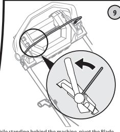
While standing behind the machine, pivot the Blade Control Handle against the premium drive control.
